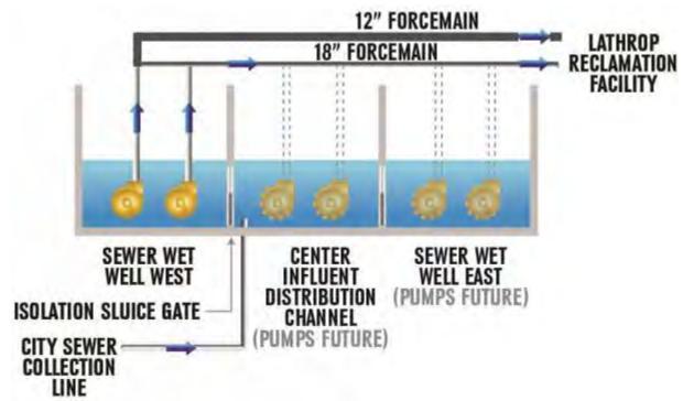
Figure 7-6: Collection Area Sewer Lift Station A1 Site Plan View
