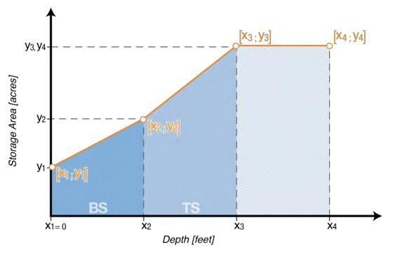
Figure 2-4: Schematic Lake Storage Capacity Graph
