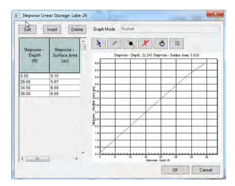
Figure 2-3: View of XPSWMM Input Data for Lake Storage Capacity
