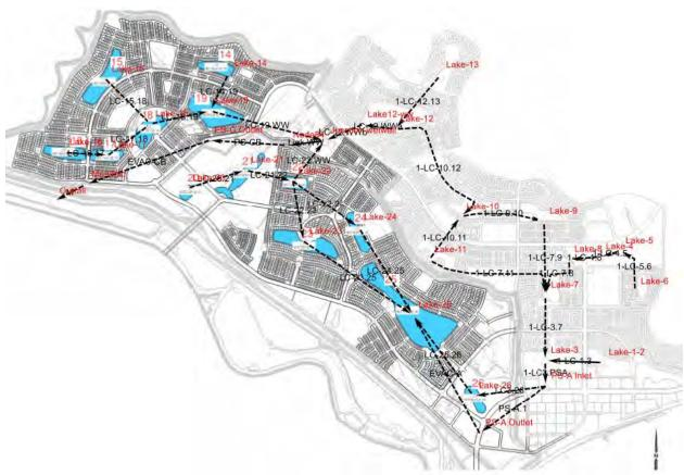
Figure 2-1: Example plan View of XPSWMM Model for phase 2
