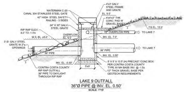
Figure 2-2: Typical Lake Outfall Structure for 36" Equalizer Pipes
