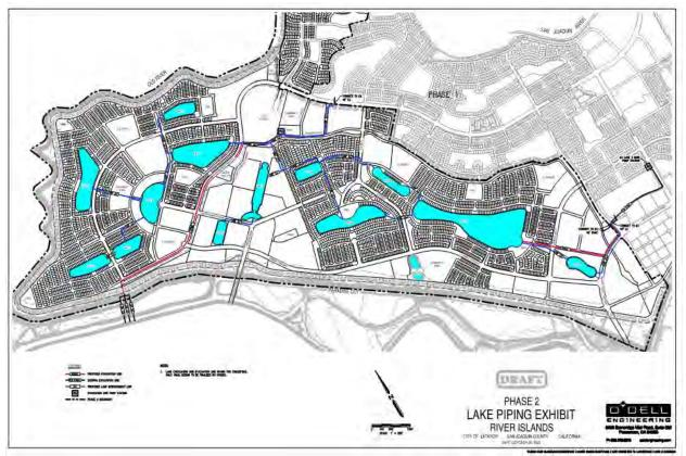
Figure 2-6: Lake interconnection pipe and pump station connection layout
