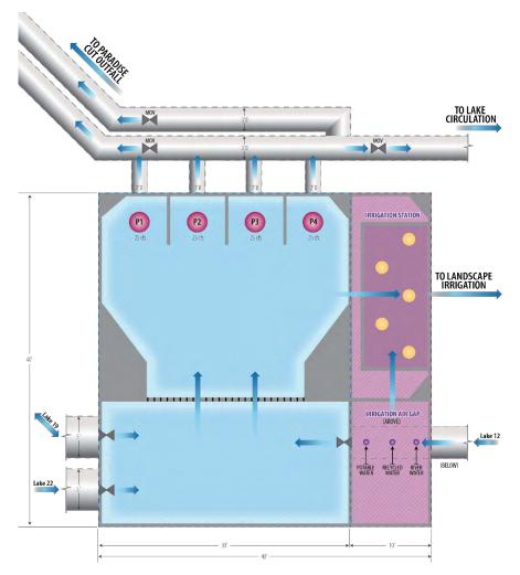
Figure 1-5: Schematic plan view of the Phase 2 pump station.
