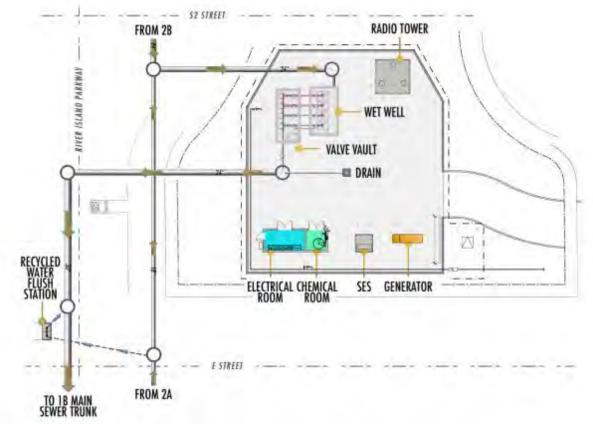
Figure 7-3: Collection Area Sewer Lift Station A1 Site Plan View
