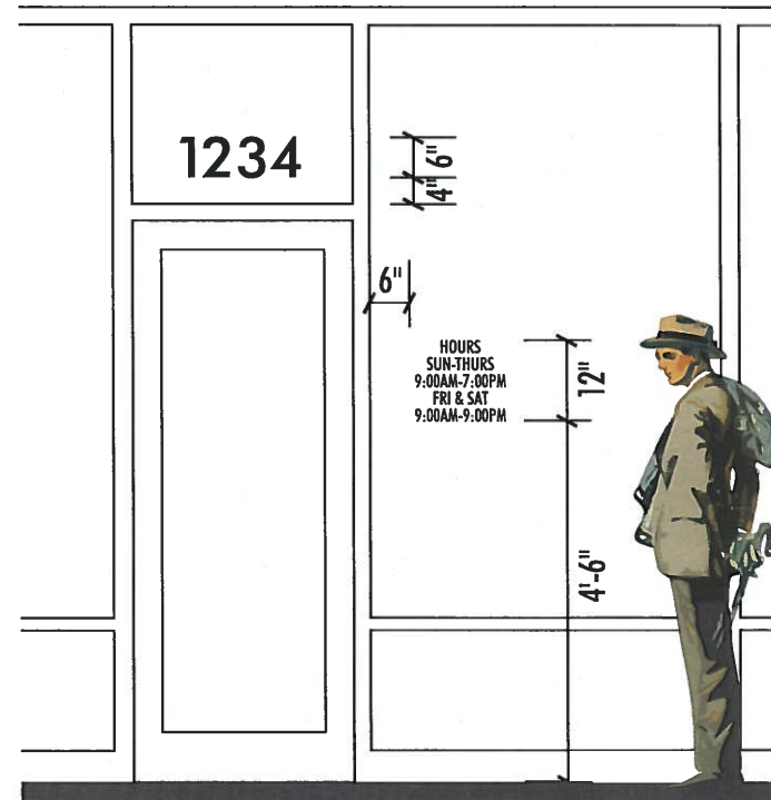
SCALE: 3/8" = 1'-0" TYPICAL FRONT ENTRY ELEVATION
