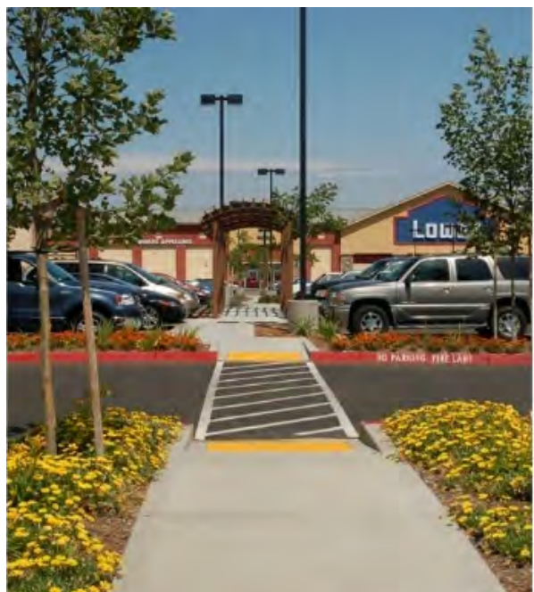
Photo Example 3 Pedestrian/bicycle safe crossing
