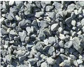
1 1/2 Inch Crushed stone
