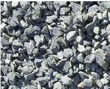
1 1/2 Inch Crushed stone
