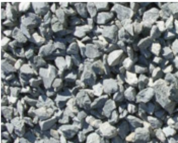
1 1/2 Inch Crushed Stone
