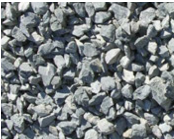
1 1/2 Inch Crushed stone
