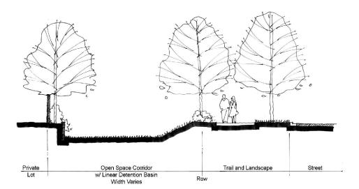
Figure 3-42: Conceptual Linear Detention Basin
