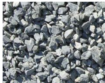
1 1/2 Inch Crushed stone
