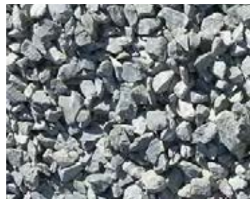
1 1/2 Inch Crushed stone
