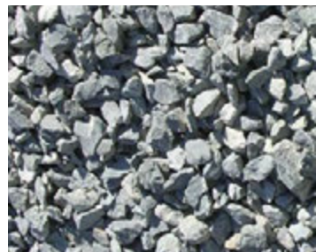
1 1/2 Inch Crushed stone
