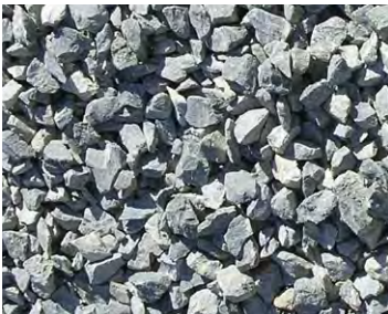
1 1/2 Inch Crushed stone
