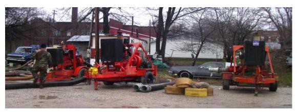
Figure 3.3 Portable pumps supplied by the Corps of Engineers during an emergency.
