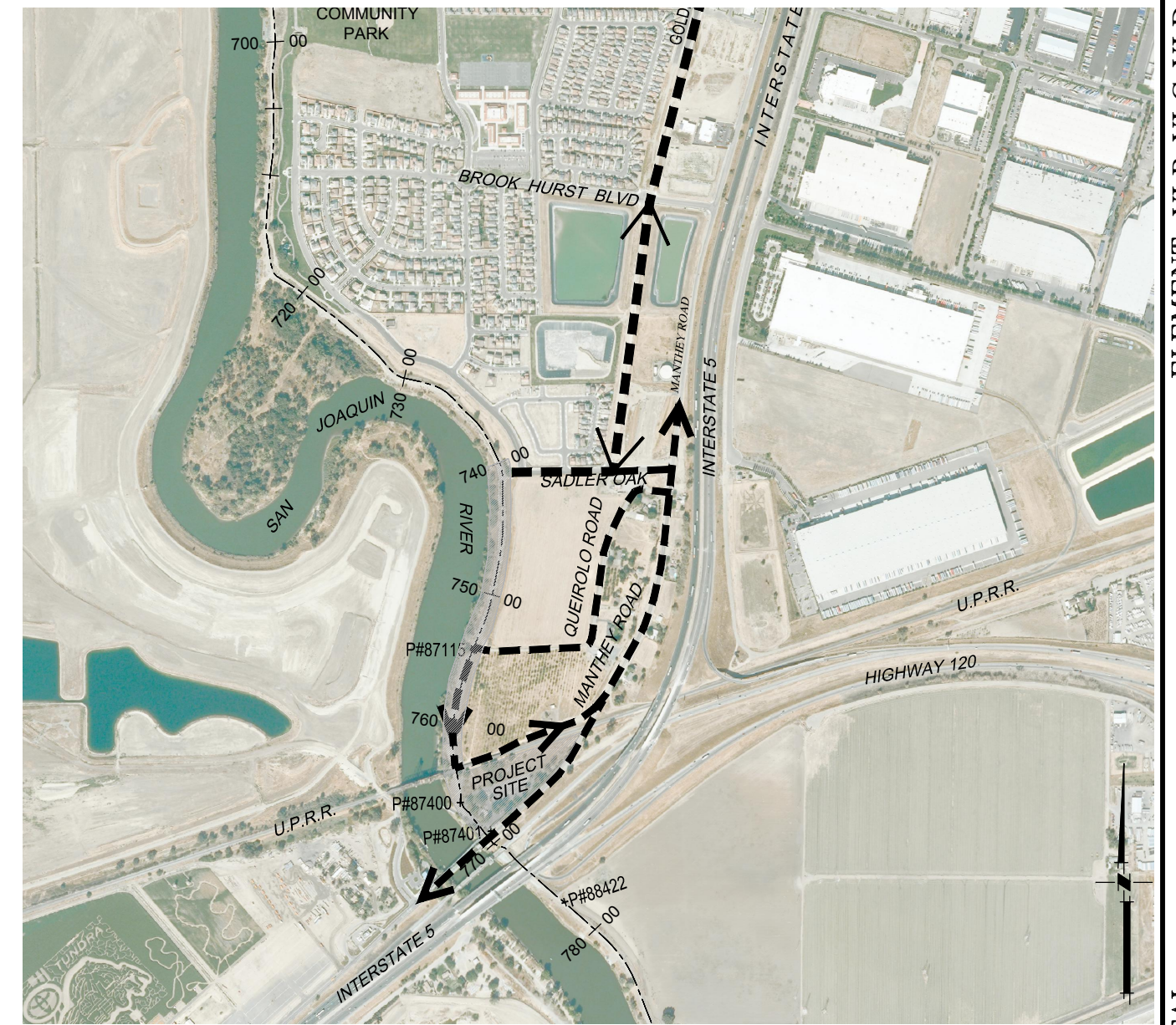
HAUL ROUTE & CONTROL POINTS 1"=600' INDICATES HAUL ROUTES TO BE USED BY CONTRACTOR
