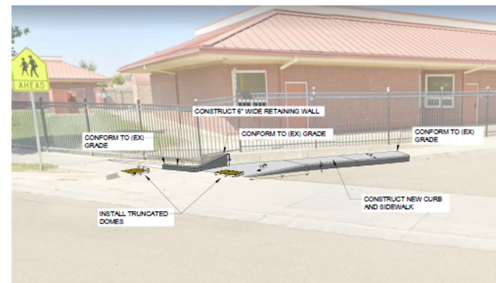
GOLDEN SPIKE TRAIL - NORTHERLY RAMP IMPROVEMENTS (N.T.S.)
