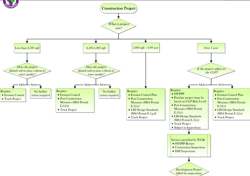
Stormwater Inspection Flow Chart 2014.vsd 8/19/2014 KMG
